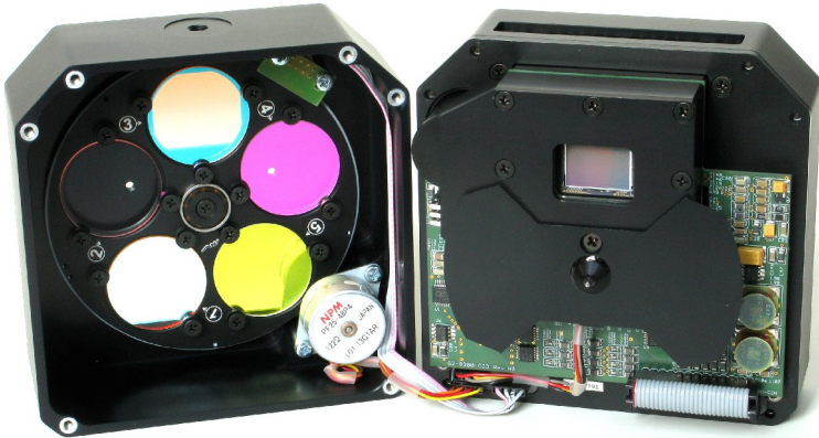
Illustration 14: Filters can be exchanged after removing of the camera front cover
