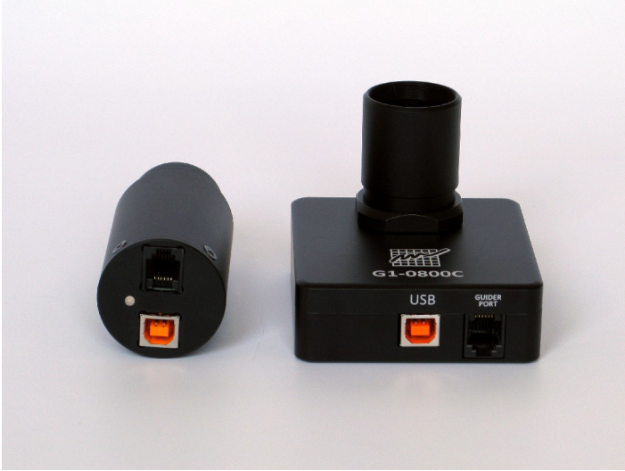
Illustration 5: Bottom side of the G0 and G1 camera heads with USB and Autoguider connectors
